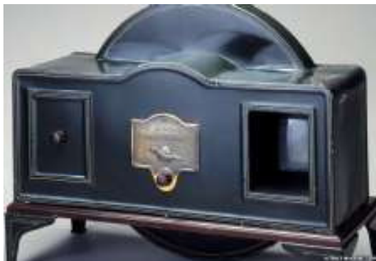
Fig 5.1 The Baird 'Televisor' - The First Commercial Television Set to Receive the 30-line Pictures (1929-1935)
